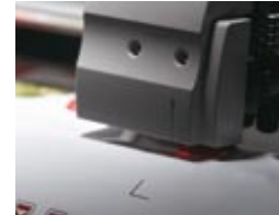
A light pointer easily adjusts the head position to the crop marks.
